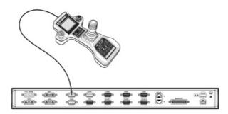
The emergency stop button on the MCUlite-2, MCU5 or MCU W has a dedicated circuit that is fed directly into the rear of the UCC controller. These connectors are then integrated to the CMM's emergency stop system in the Renishaw servo power amplifiers or UCC controller. If non-Renishaw servo power amplifiers are used then it is the integrators responsibility to connect the MCU E-STOP switch into the emergency stop system.
